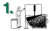
Operator inserts key and turns to "UP" position. When ram moves to up position the door can be opened.
